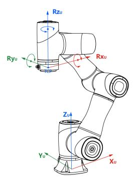
Figure 2.17 The default User coordinate system of CR3 robot
