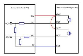
Figure 3.10 End I/O connection
