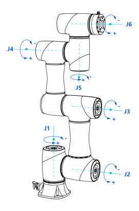
Figure 2.14 Joint coordinate of a CR3 robot
