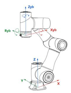
Figure 2.15 Base coordinate system of CR3 robot
