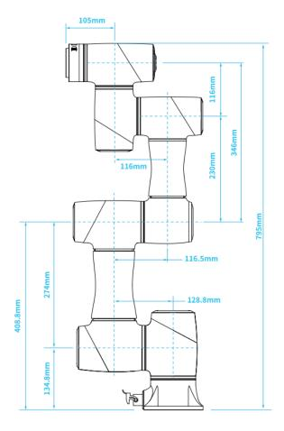
Figure 2.2 Robot body size
