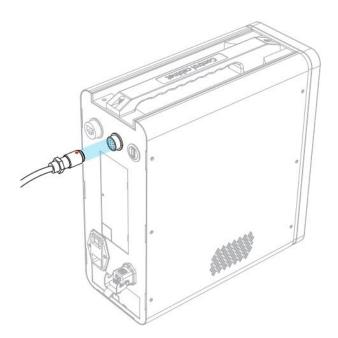
Figure 4.4 Connecting emergency stop switch
