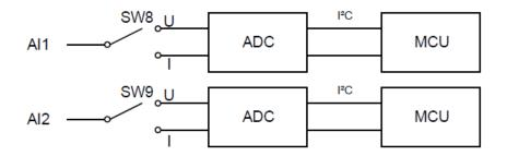
Figure 3.6 Simple analog input circuit
