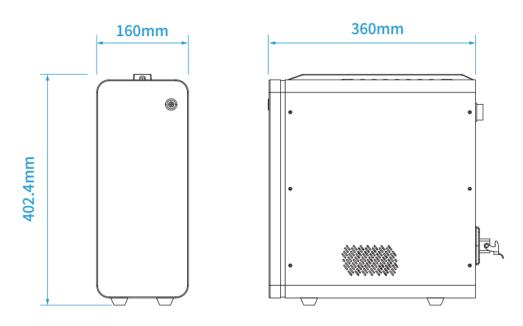
Figure 2.3 Controller size
