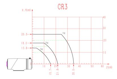
Figure 2.6 End-effector load curve
