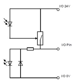
Figure 3.5 Simple digital output circuit
