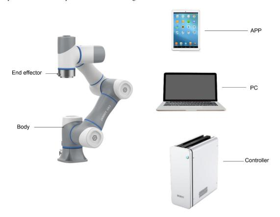
Figure 2.1 Robot system
