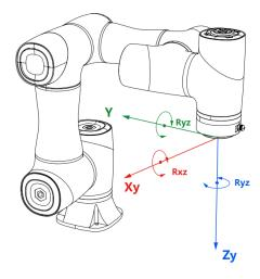
Figure 2.16 The default Tool coordinate system of CR3 robot
