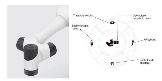
Figure 2.21 Keys on robot
