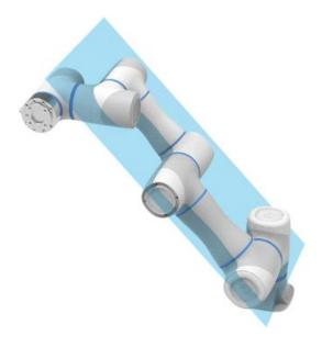
Figure 2.20 Elbow singularity point
