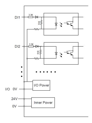
Figure 3.4 Simple digital input circuit
