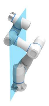
Figure 2.19 Shoulder singularity point
