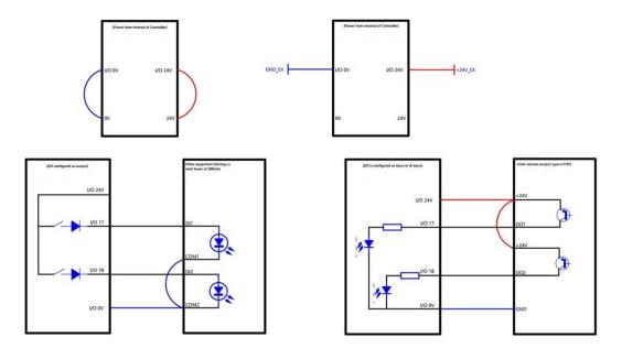
Figure 3.3 Controller I/O Connection
