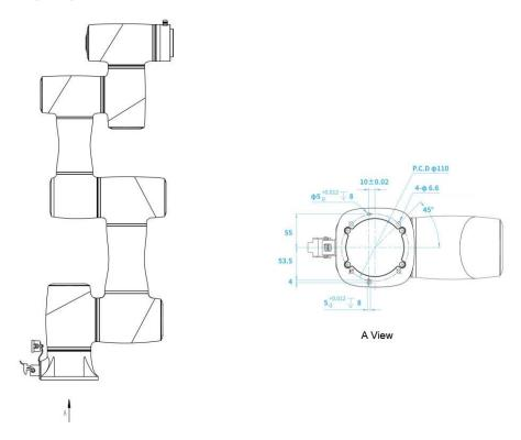
Figure 4.2 Robot base size
