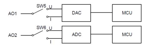
Figure 3.7 Simple analog output circuit
