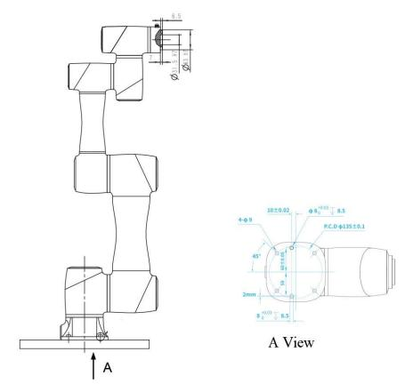
Figure 4.2 Robot base size
