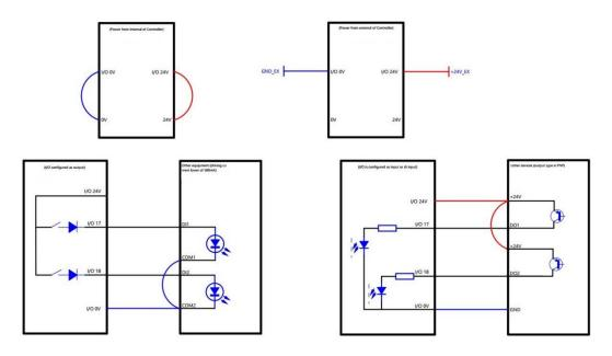
Figure 3.3 Controller I/O Connection
