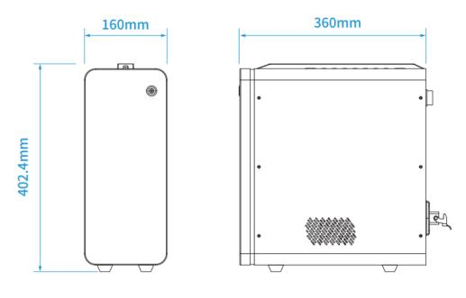
Figure 2.3 Controller size
