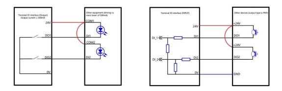
Figure 3.10 End I/O connection
