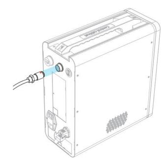
Figure 4.4 Connecting emergency stop switch
