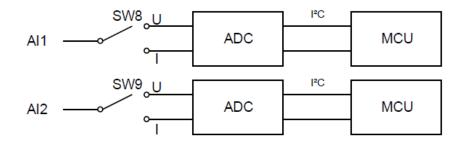
Figure 3.6 Simple analog input circuit
