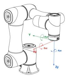
Figure 2.15 The default Tool coordinate system of CR7 robot
