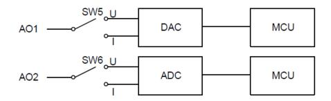
Figure 3.7 Simple analog output circuit
