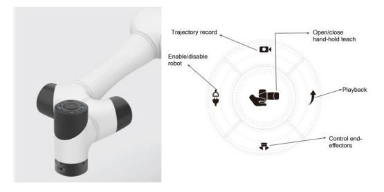
Figure 2.20 Keys on robot
