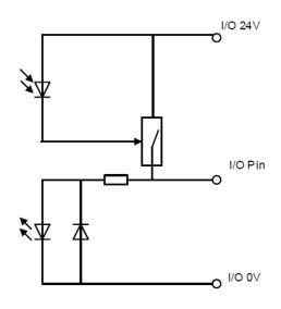
Figure 3.5 Simple digital output circuit
