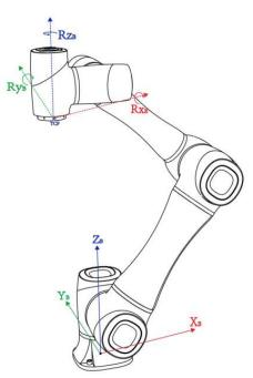
Figure 2.14 Base coordinate system of CR7 robot
