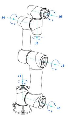
Figure 2.13 Joint coordinate of a CR7 robot
