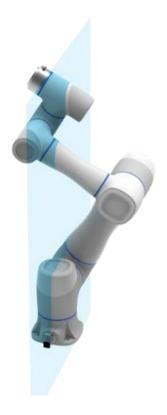
Figure 2.18 Shoulder singularity point
