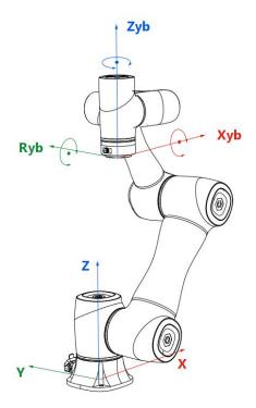
Figure 2.16 The default User coordinate system of CR7 robot
