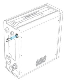
Figure 4.5 Connecting WiFi module
