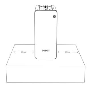
Figure 4.1 Installation space requirement
