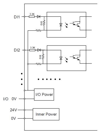
Figure 3.4 Simple digital input circuit
