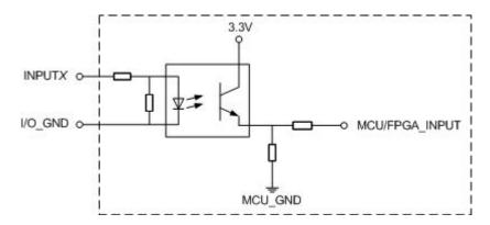
Figure 3.4 Simple digital input circuit
