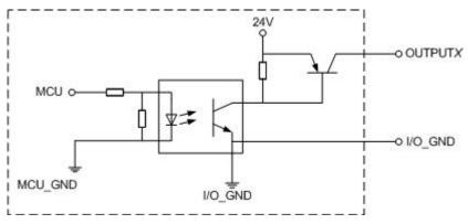
Figure 3.5 Simple digital output circuit
