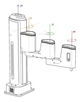
Figure 2.9 Joint coordinate of a M1 Pro robot
