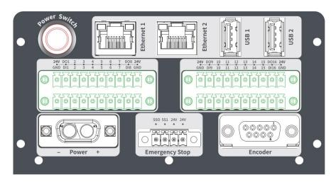
Figure 3.1 Interface board of the base
