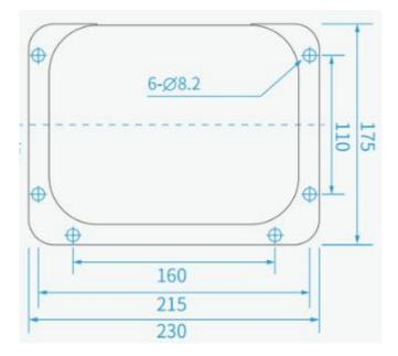
Figure 4.1 Robot base size
