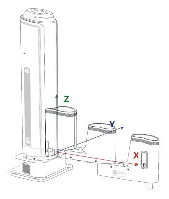
Figure 2.10 Base coordinate system of M1 Pro robot
